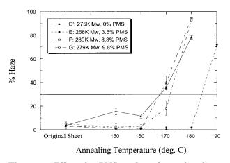
Figure 3 Effect of % PMS on the % haze of medium Mw sPS sheets. (Note: The D' data points were obtained by interpolation from the data points of samples D and H.)
