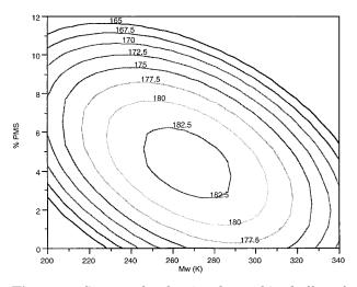
**Figure 5** Contour plot showing the combined effect of Mw and % PMS on the clear-to-hazy transition temperature of sPS sheets.
