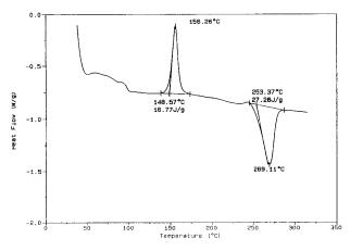
**Figure 1** A typical DSC scan for SPS sheets (heating rate: 20°C/min).
