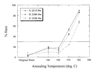
Figure 2 Effect of Mw on the % haze of sPS homopolymer sheets.
