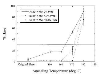
Figure 4 Effect of % PMS on the % haze of low Mw sPS sheets.
