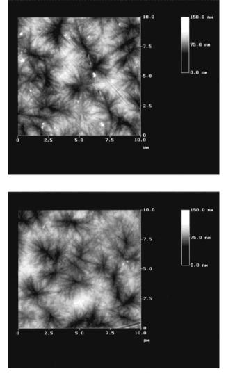
**Figure 6** AFM pictures showing spherulite-like structures on the surfaces of both a clear (top, sample A annealed at 150°C) and a hazy (bottom, sample A annealed at 180°C) sPS sheet.
